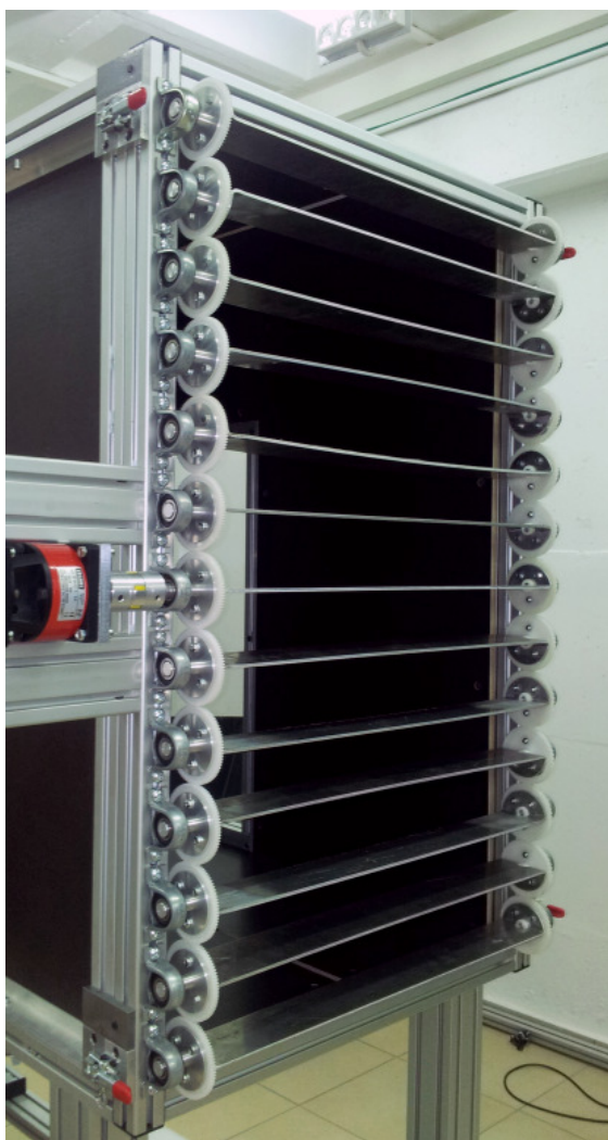
Figure 1. Photograph of the louver system attached to downstream test section for the present experiments with the radial diffuser removed (vanes fully open).
